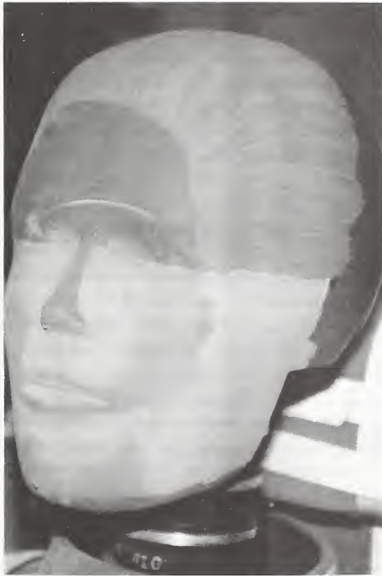
FIGURE 23 -- Left Side View of Chalk Removal Pattern for System I
